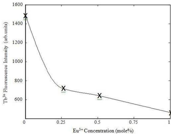
**Fig. 2. Intensity of Tb<sup>3+</sup> (<sup>5</sup>D<sub>4</sub> → <sup>7</sup>F<sub>5</sub>) transition co-doped with Eu<sup>3+</sup>: sodium fluoroborate glass**
