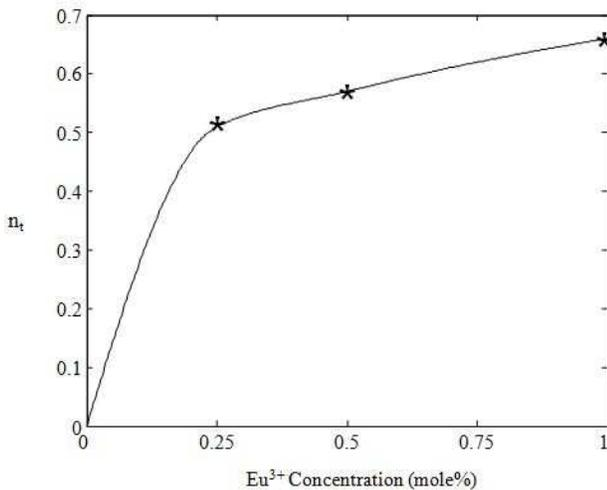
**Fig. 3. Energy transfer efficiencies of Tb<sup>3+</sup> co-doped with Eu<sup>3+</sup> : sodium fluoroborate glass**
